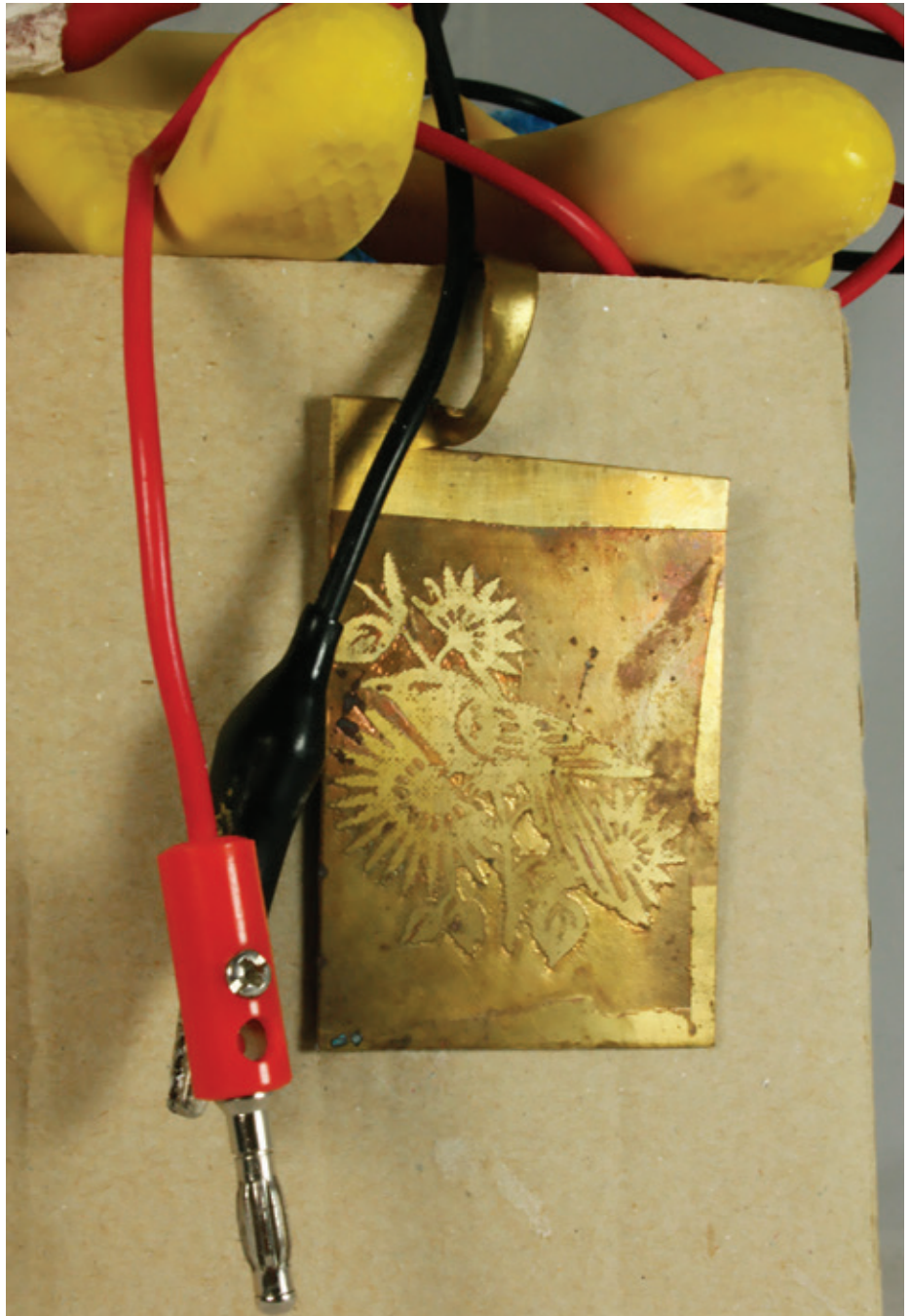
Electrolytic etching a test piece from Dauvit's 2010 Crossings Conference workshop. Photo: Poppy Porter
